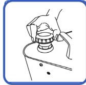
3. Open the filler safety cap slightly to allow the remaining steam to release.
