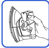
2. Press the steam button on the iron handle until the pressure drops to zero.
